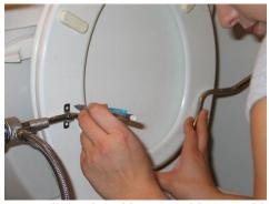
4. Hold the hoop so the ball nozzle is approximately perpendicular to the center of the toilet seat. This insures that the nozzle will track on the
